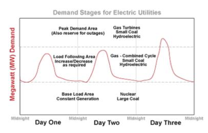
have spinning generators but are not loaded, are brought instantly online. Gas turbines — essentially jet plane engines connected to a generator — are also able to add generating capacity in a very short time.
