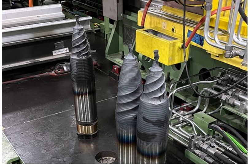
ProPublica/X Mangled artillery shells produced at General Dynamics plant in Mesquite, Texas
