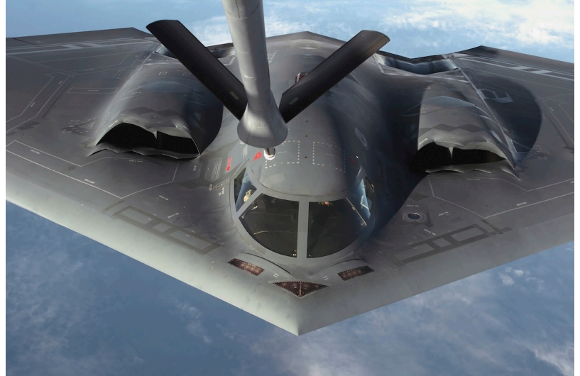
Stocktrek Images/iStock/Getty Images Plus B-2 Spirit bomber approaching a KC-135 Stratotanker to refuel
