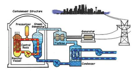
**Pressurized water reactor:** The primary loop (red) of a PWR keeps water under high pressure to prevent boiling. It heats low-pressure water in the secondary loop (blue) without transmitting radioactivity in the process.
